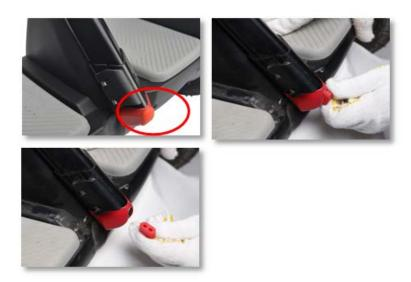
Loosen the quick release and then remove the knee bar assembly
